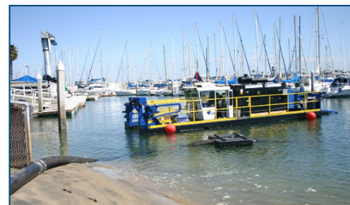
A Model 5012 HP removes sand from a large marina in California.
